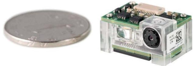
With its compact dimensions and integrated decoder, the N3680 makes it easy to incorporate high performance scanning into your designs.
