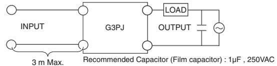
2. The G3PJ with Rated Load Voltage of 100 to 480 VAC (5□□B model)
