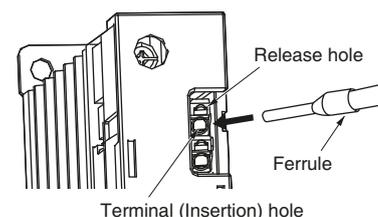
If a wire is difficult to connect because it is too thin, use a flat-blade screwdriver in the same way as when connecting stranded wire.
