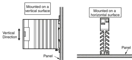
**Note:** Make sure that the load current is 50% of the rated load current when the G3PJ is mounted horizontally. For details on close mounting, refer to the related information under performance characteristics. Mount the G3PJ in a direction so that the markings read naturally.
