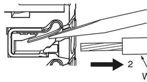
3. Remove the flat-blade screwdriver from the release hole.
