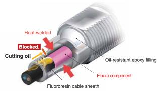
Note: With Proximity Sensors, there is limited space available to block the ingress of cutting oil. The usage of cables with fluororesin outer sheaths enables limiting the ingress path from the cable to one point, that is, the surface between the cable and the structural components.
