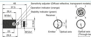
Operation indicator (orange) Stability indicator (green) Receiver Emitter Optical axis
