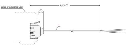
\*4-dia. cable with 2 conductors, Standard cable length: 2 m (Conductor cross-section: 0.2 mm<sup>2</sup> (AWG24), Insulation diameter: 1.1 mm)
