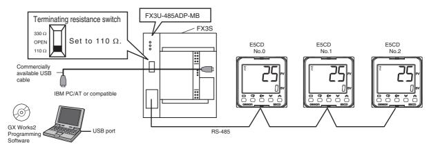
Note: Refer to the GX Works2 Installation Instructions (BCN-P5713) for information on installing the GX Works2 and to the GX Works2 Version 1 Operating Manual (Common) (SH-080779ENG) for information on installing the USB driver.
