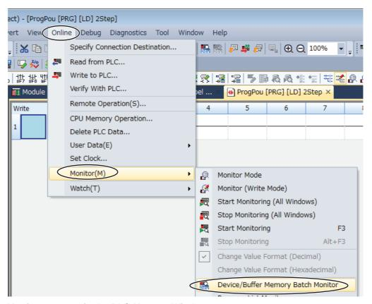
(2) Monitor memory in the PLC Memory Window. Enter D0 in the Device Name Box and click the Start Monitoring Button to start monitoring.
