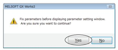
(2) Messages will be displayed asking whether or not to add labels for mounted Modules. One message will be displayed for each mounted Module.
