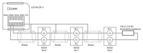
Note: 1 The maximum transmission distance is 50 m for the CP1W-CIF11 and 500 m for the CP1W-CIF21.
