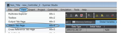
(b) If you enter the name of the variable that you created in step 2 in the Name column of the Watch (Table) 1 Tab Page displayed at the bottom of the window, the contents of D000 to D038 will be displayed.
