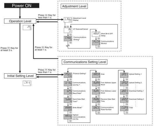
\* These parameters are displayed regardless of the setting of the Protocol Setting parameter.
