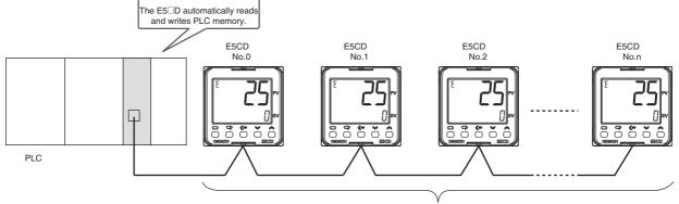
Up to 32 E5□D Controllers on one communications line (up to 16 Controllers for a Mitsubishi FX-series PLC)
