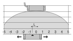
5 mm misalignment tolerance after setting
