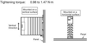
Note: Make sure that the load current is 50% of the rated load current when the G3PJ is mounted horizontally.
