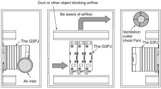
Note: 1. If the air inlet or air outlet has a filter, clean the filter regularly to prevent it from clogging to ensure an efficient flow of air.
