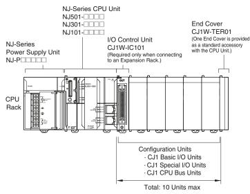
Even though the NJ-Series Controllers do not have Backplanes, the term "slot" still used to refer to the location of Units. Slot numbers are assigned in order to Units from left to right on the CPU Rack (slot 0, slot 1, slot 2, etc.).
