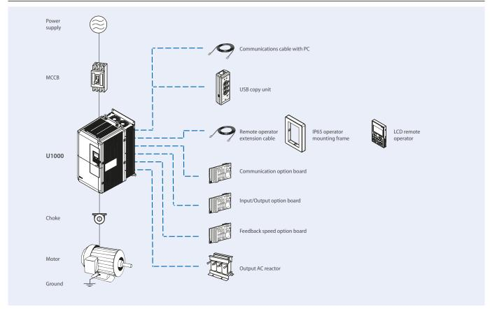
$\textbf{Note:} \quad \textbf{U1000 includes EMC filter, input AC reactor, regenerative converter and frequency drive.}$
