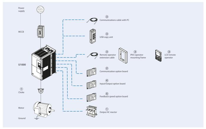
Note: U1000 includes EMC filter, input AC reactor, regenerative converter and frequency drive.
