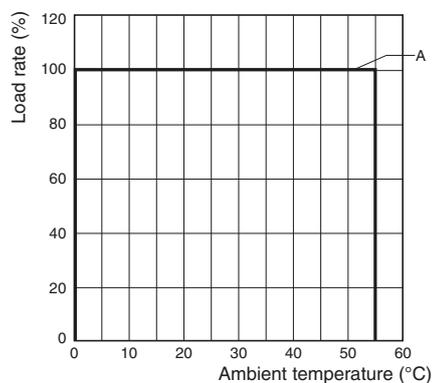
A: For standard mounting, face-up mounting, stationary mounting
