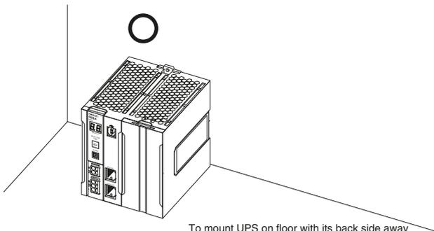
To mount UPS on floor with its back side away from you, mount it so that its back side is in contact with wall. (Because PCB is partially exposed in its back side, and UPS may be affected by static electricity for that reason.)
