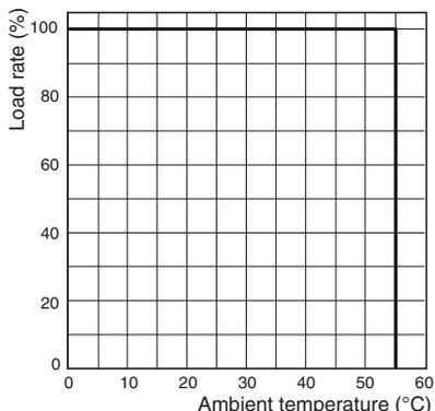
**Contact mounting (Less than 15 mm space between the left and right)**
