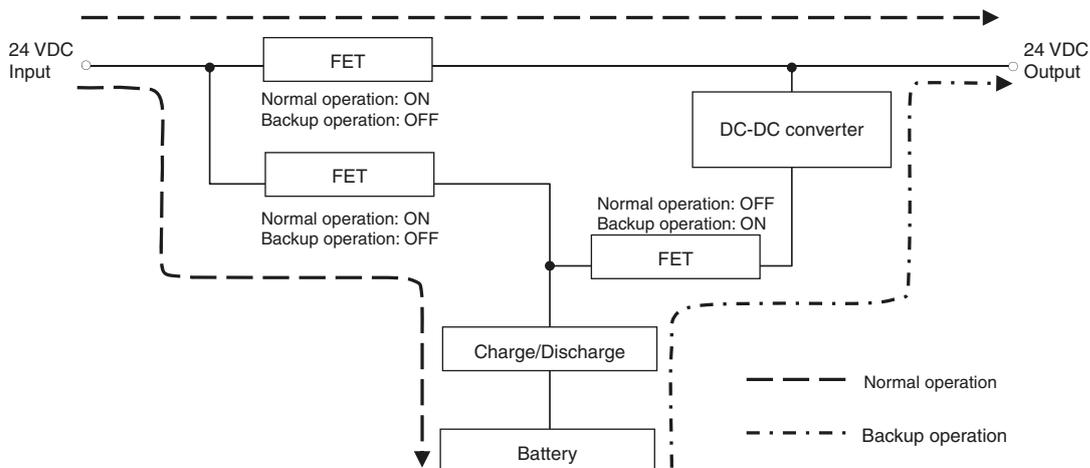
\* In normal operation, 24 VDC is output as-is for charging the battery and from the input power supply. If 24 VDC from the input power supply drops, the operation automatically switches to backup operation, and 24 VDC is output from the battery.
