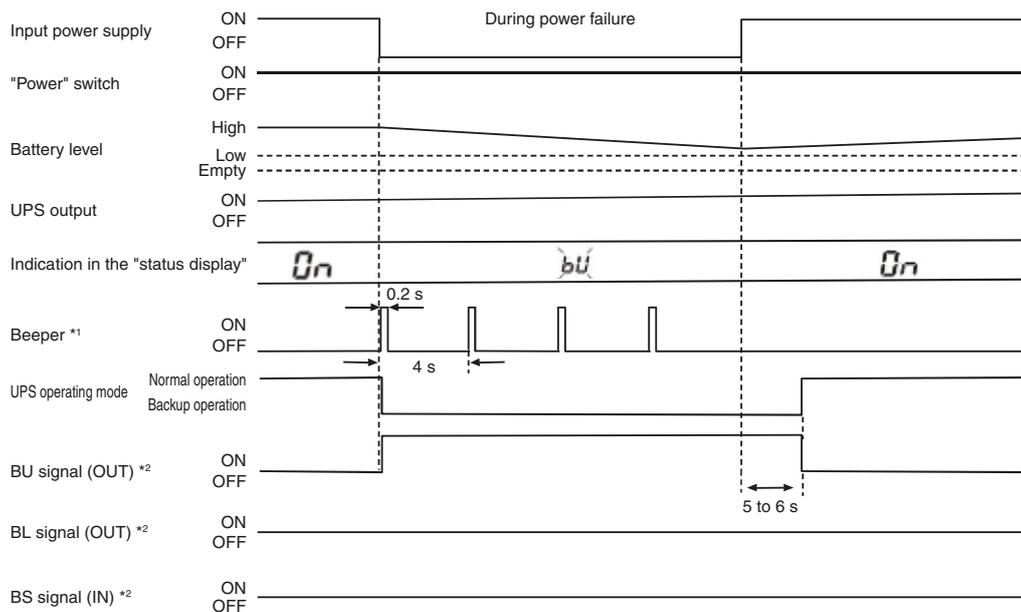
\*1. "Disable beeper" is set by factory default. When "Disable beeper" is set, the buzzer does not sound during backup operation. For details, refer to 4-4 UPS operation mode settings.
