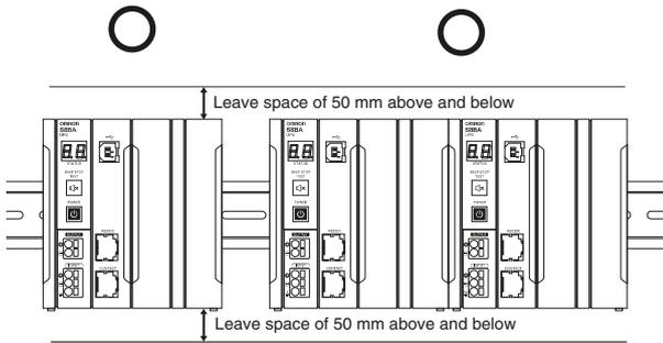
To install devices other than the UPS to both sides, install them by leaving a space specified by each device off the UPS.
