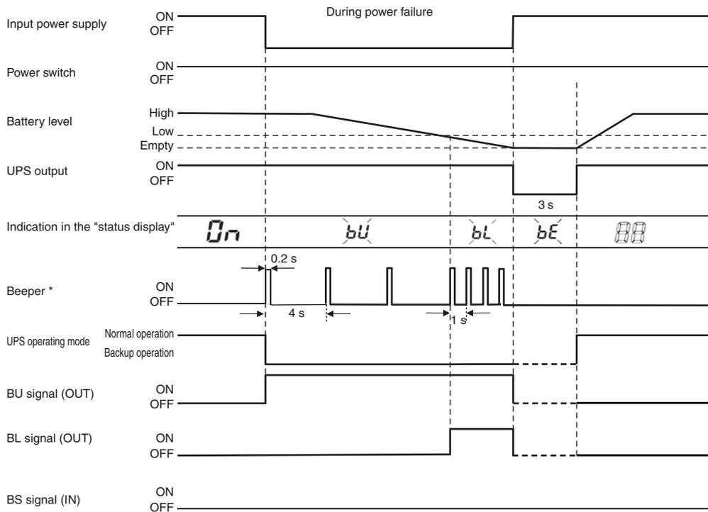
\* "Disable beeper" is set by factory default. Even when "Disable beeper" is set, the buzzer sounds at startup.
