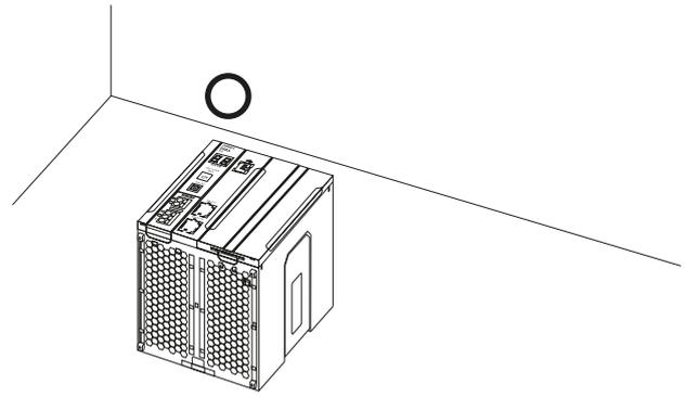
To mount UPS on floor with its top side away from you, mount it so that its top side is 50 mm or more off wall.
