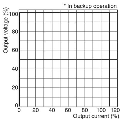
**Note:** 1. In backup operation, the output voltage drops at a load rate of 110% or higher.
