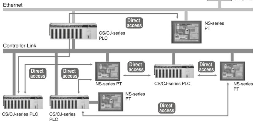
**You may want to transfer screens to a PT through the PLC without changing computer connections or transfer a ladder program to the PLC through the PT by using the Ethernet or Controller Link.**
