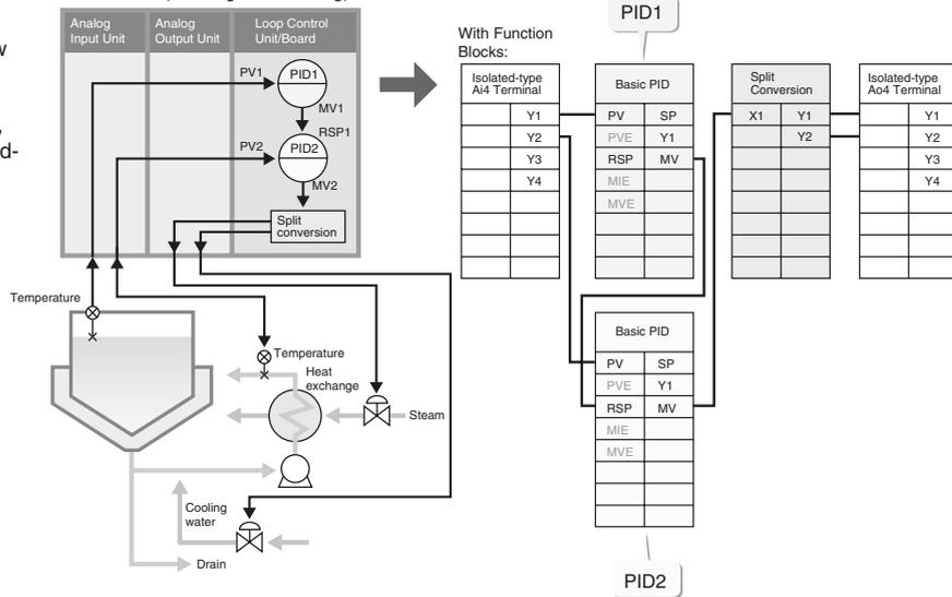
**PLC-based Process Control Application Examples**
