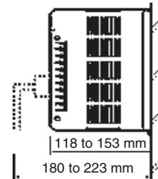
**Note:** I/O Connecting Cables require sufficient space to maintain the min. bending radius.
