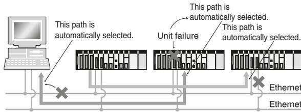
The CS1D-ETN21D and CS1D CPU Unit version 1.1 or higher are required for a duplex Ethernet network.
