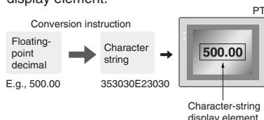
The new CS1 can convert ASCII character strings read from measurement devices by serial communications to floating-point decimal data for use in data processing.
