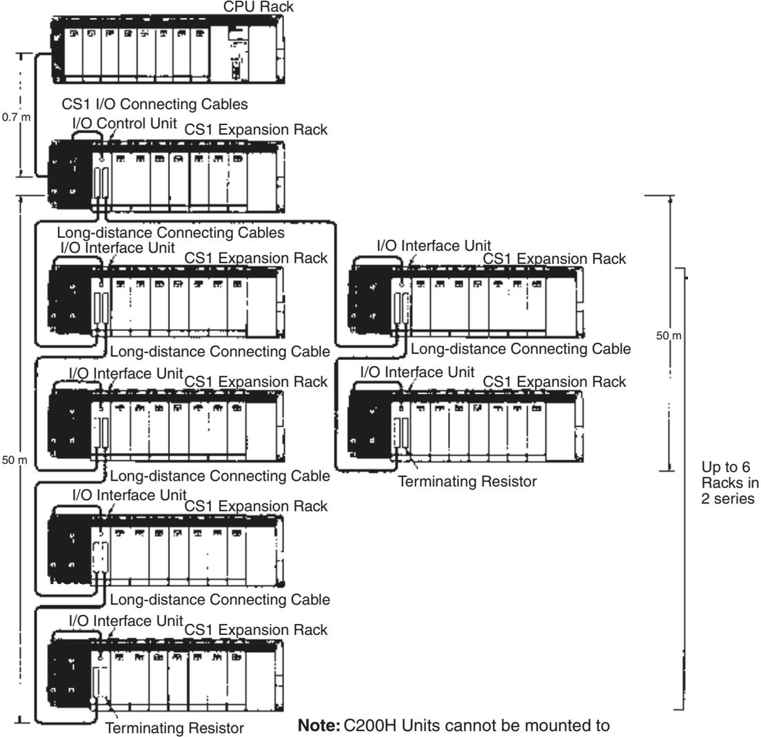
**Note:** C200H Units cannot be mounted to Long-distance Expansion Racks. (They can be mounted to the CS1 Expansion Rack with the I/O Control Unit mounted.)
