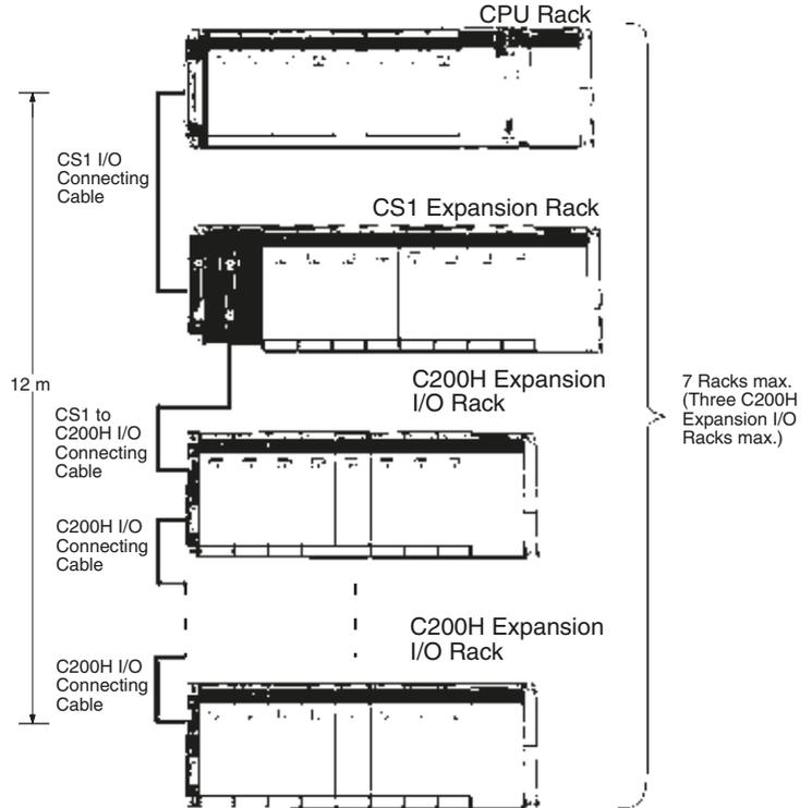
**CPU Rack with CS1 Long-Distance Expansion Racks**
