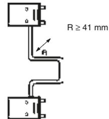
CS1 to C200H I/O Connecting Cable (Cable diameter: 5.1 mm)
