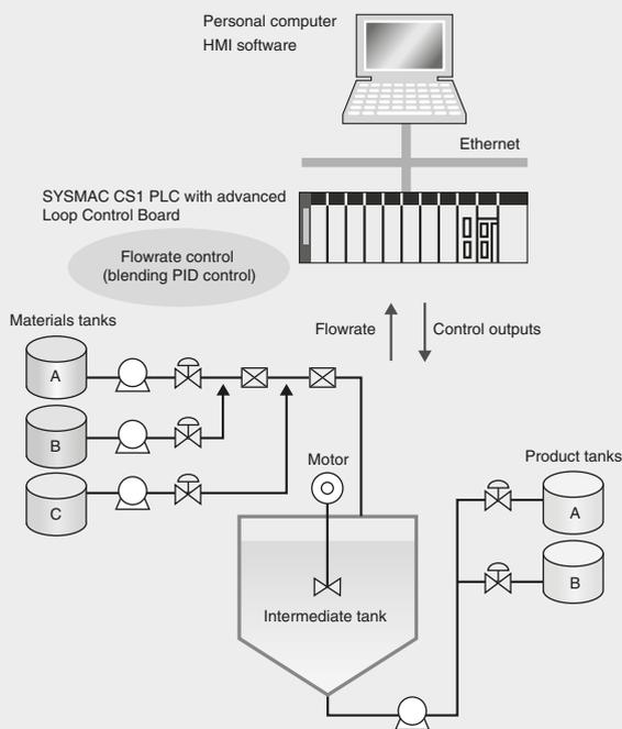
● Batch Control in a Chemical Plant
