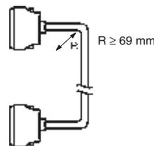
C200H I/O Connecting Cable (Cable diameter: 5.1 mm)
