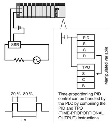
Time-proportioning PID control can be handled by the PLC by combining the PID and TPO (TIME-PROPORTIONAL OUTPUT) instructions.
