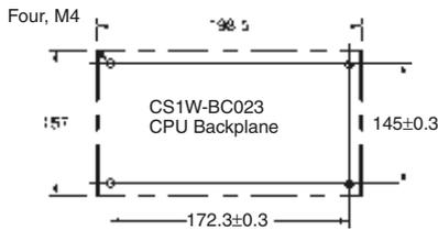
**Note:** Expansion Backplanes cannot be connected to 2-slot CPU Backplanes.
