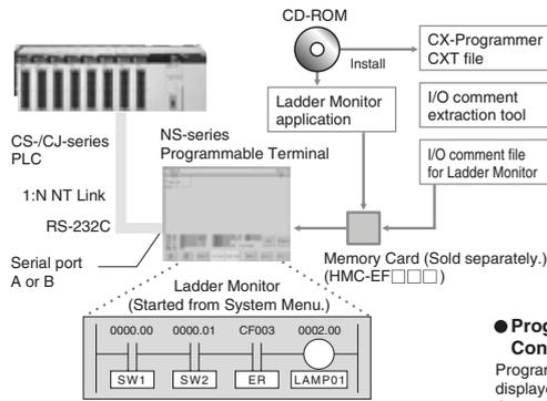
**Note:** CS- and CJ-series PLCs connected via a 1:N NT Link to serial port A or B on an NS-series Programmable Terminal can be monitored.
