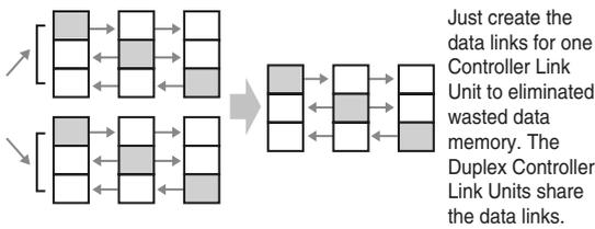
Just create the data links for one Controller Link Unit to eliminate wasted data memory. The Duplex Controller Link Units share the data links.
