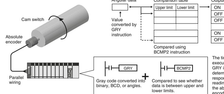
The time interval for execution by the GRY instruction is determined by the response speed for reading data from the absolute encoder.
