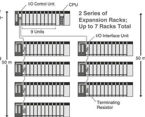
Note: C200H Units cannot be mounted on the Long-distance Expansion Racks.
