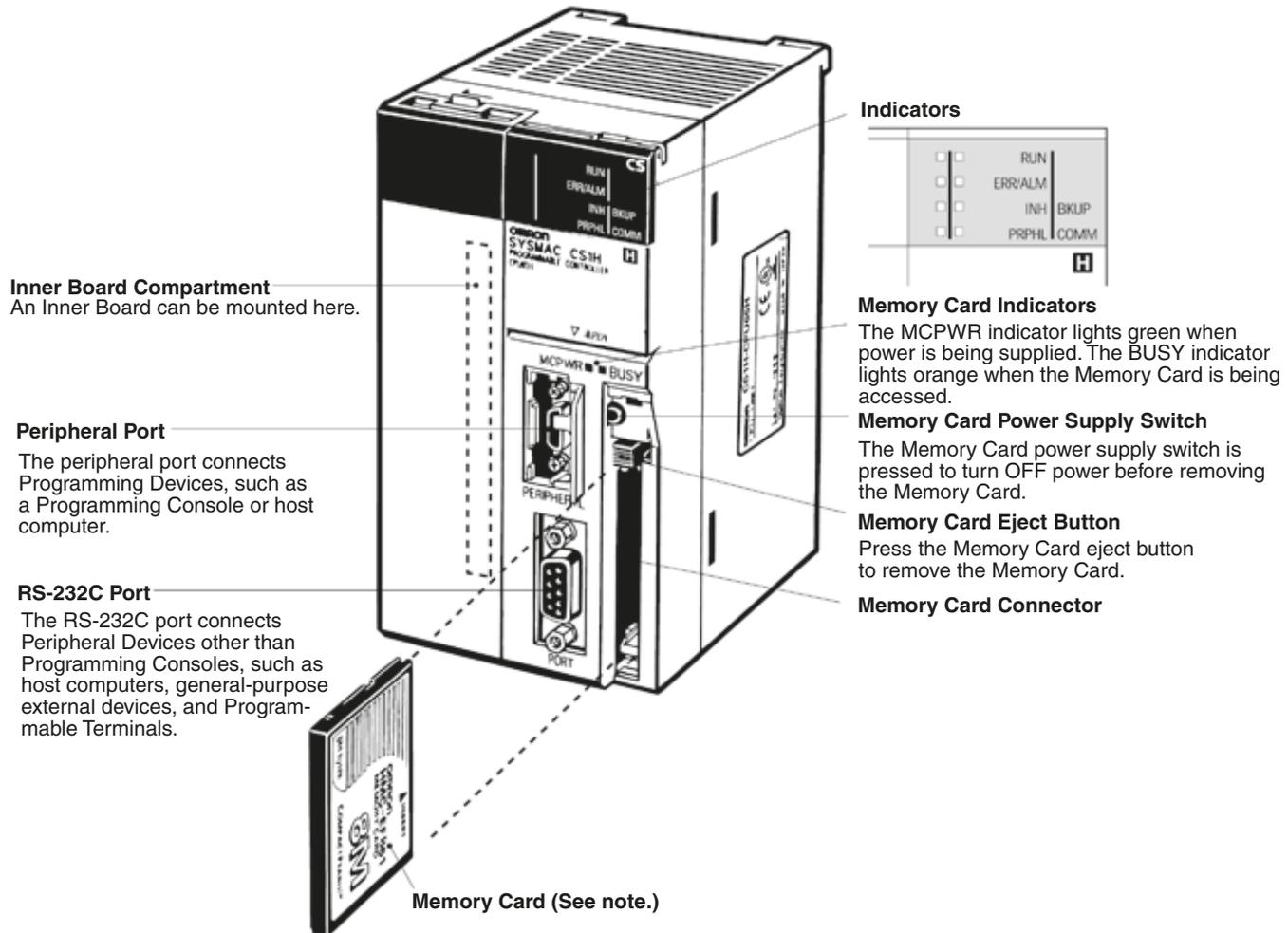
With the CS1 PLCs, Memory Cards and specified ranges of the EM Area can be used as file memory. File memory can be used to store the entire user program, I/O memory contents, and/or parameter area contents.
