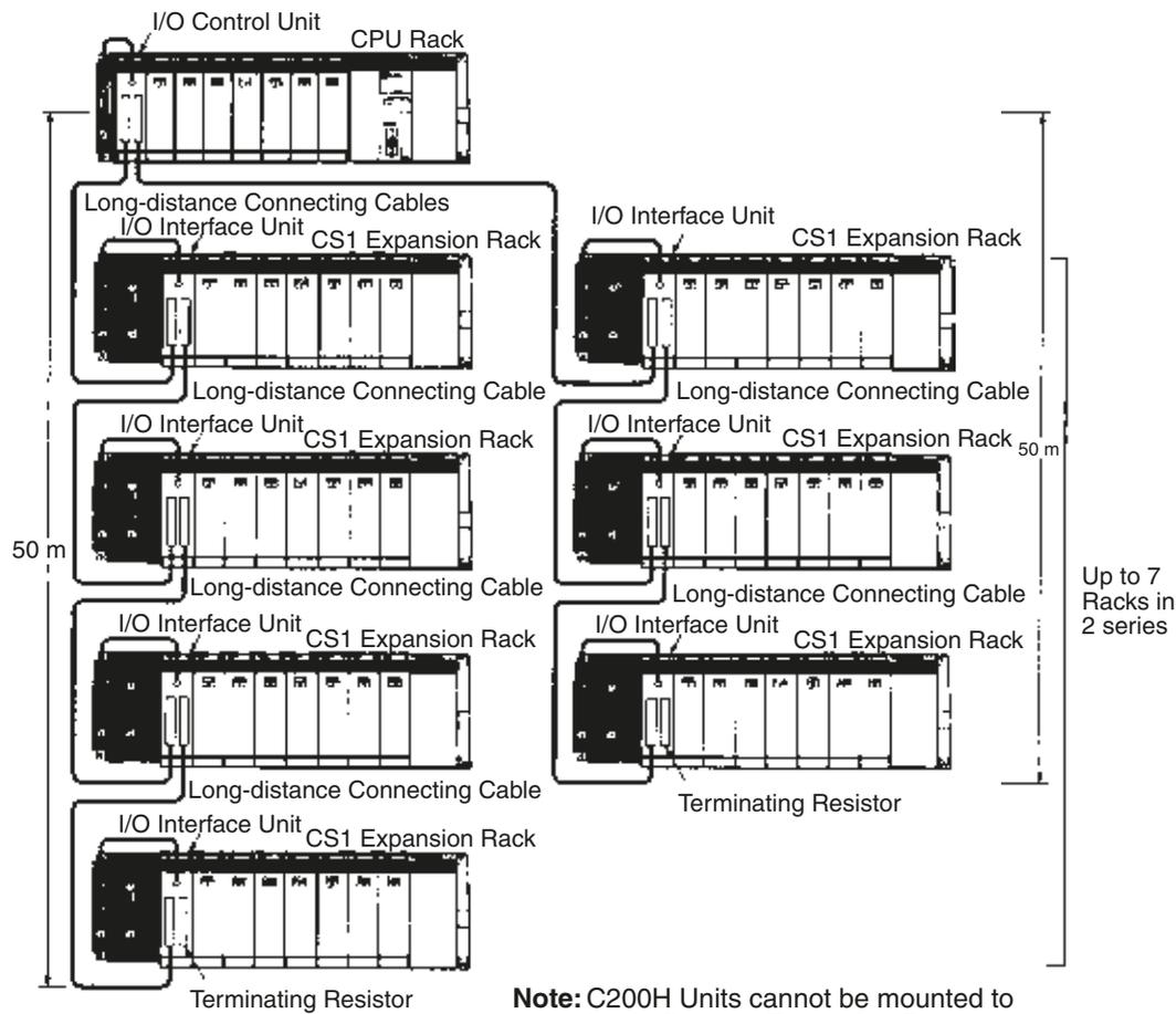
**Note:** C200H Units cannot be mounted to Long-distance Expansion Racks.
