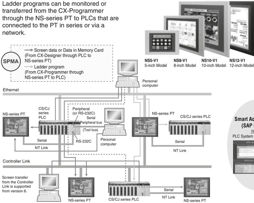
**NS-series PTs provide Smart Active Parts (SAP library) enabling direct access to data in various devices.**
