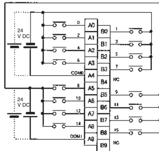
Polarity of the input power supply can be connected in either direction.
