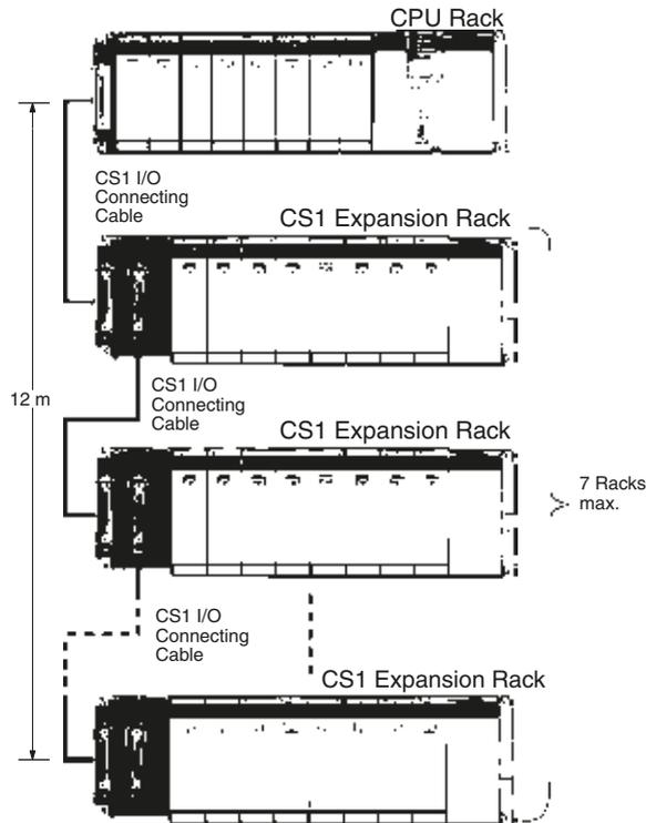
**CPU Rack with CS1 Expansion Racks and C200H Expansion I/O Racks**
