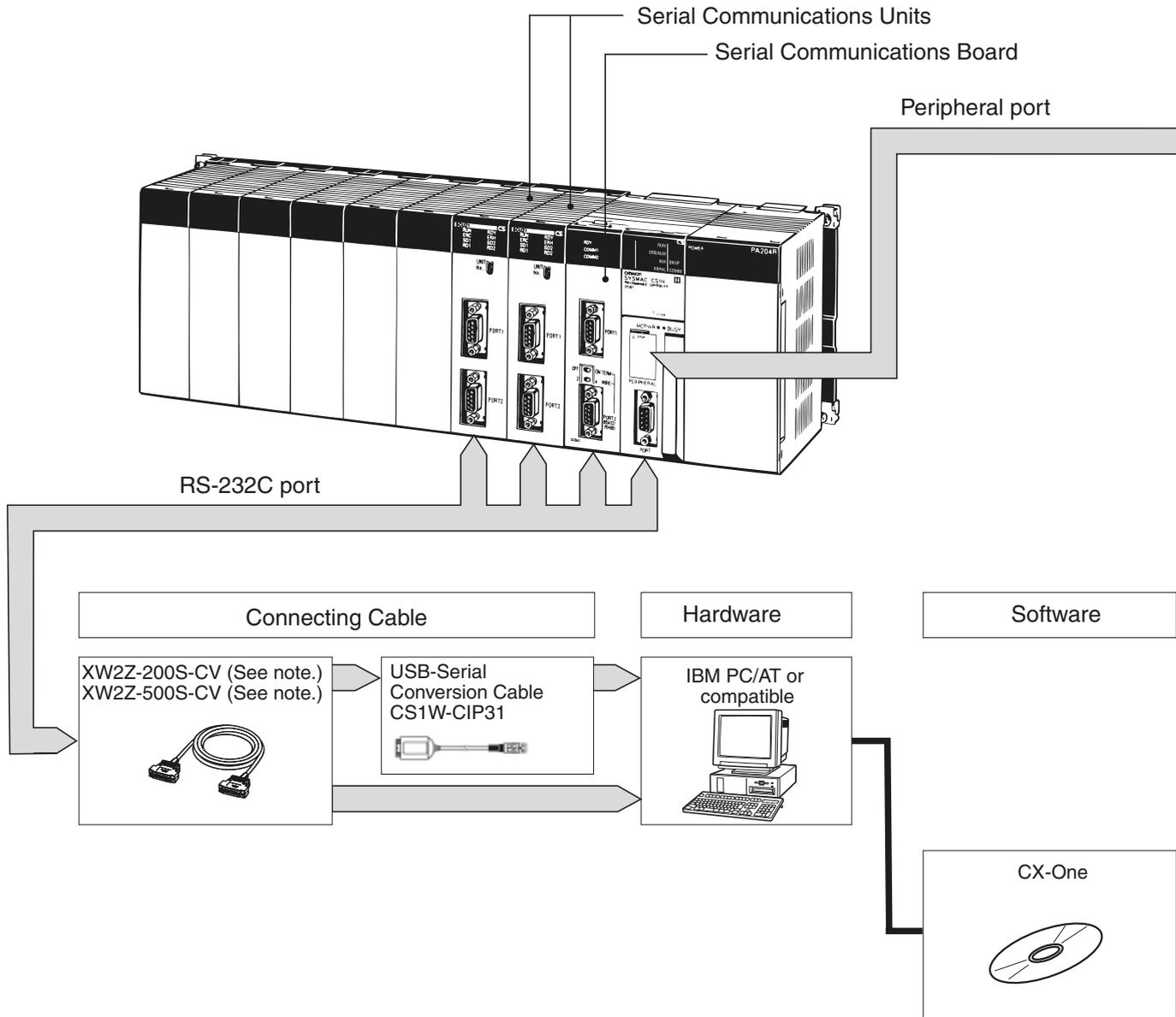
**Note:** Refer to the next page for details of cables for connecting to computers. Choose the appropriate cable for the communications mode.
