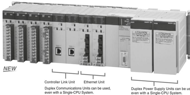
Duplex operation is possible for any or all of the following: CPU Units, Power Supply Units, and Communications Units.
